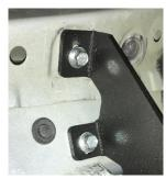
**Step 7:** There will be  $\frac{1}{2}$ " of adjustment in the (x3) mounting bracket. Adjust to desired position and tighten to (20 ft,/lbs).
