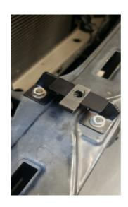
Step 3: Install the 3 supply brackets as shown above:
