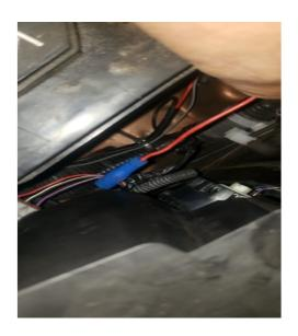
Step 7: (This is for Tundra's with the LED Glow Option). Our grille is supplied with a posi tap to tap into your marker light on the driver's side. The purple wire is located next to the battery in a plastic casing. The ground wire with the eyelet can be grounded anywhere.
