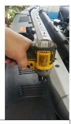
Step 1: Remove the two plastic clips on top of the radiator and the four 10mm screws on the radiator support. At this point the whole grille assembly will be removed from the truck.
