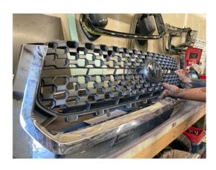
Step 2: Separate the outer shell, and the factory center of the grille.
