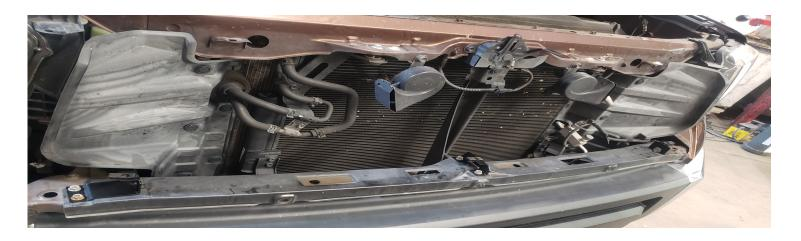
At this point then you can install the grille on those three brackets. Reach through the top holes and secure the three bolts through the grill onto those three brackets, as shown.
